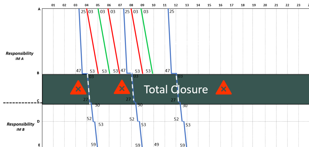
Figure 9 Total Closure between B and C
