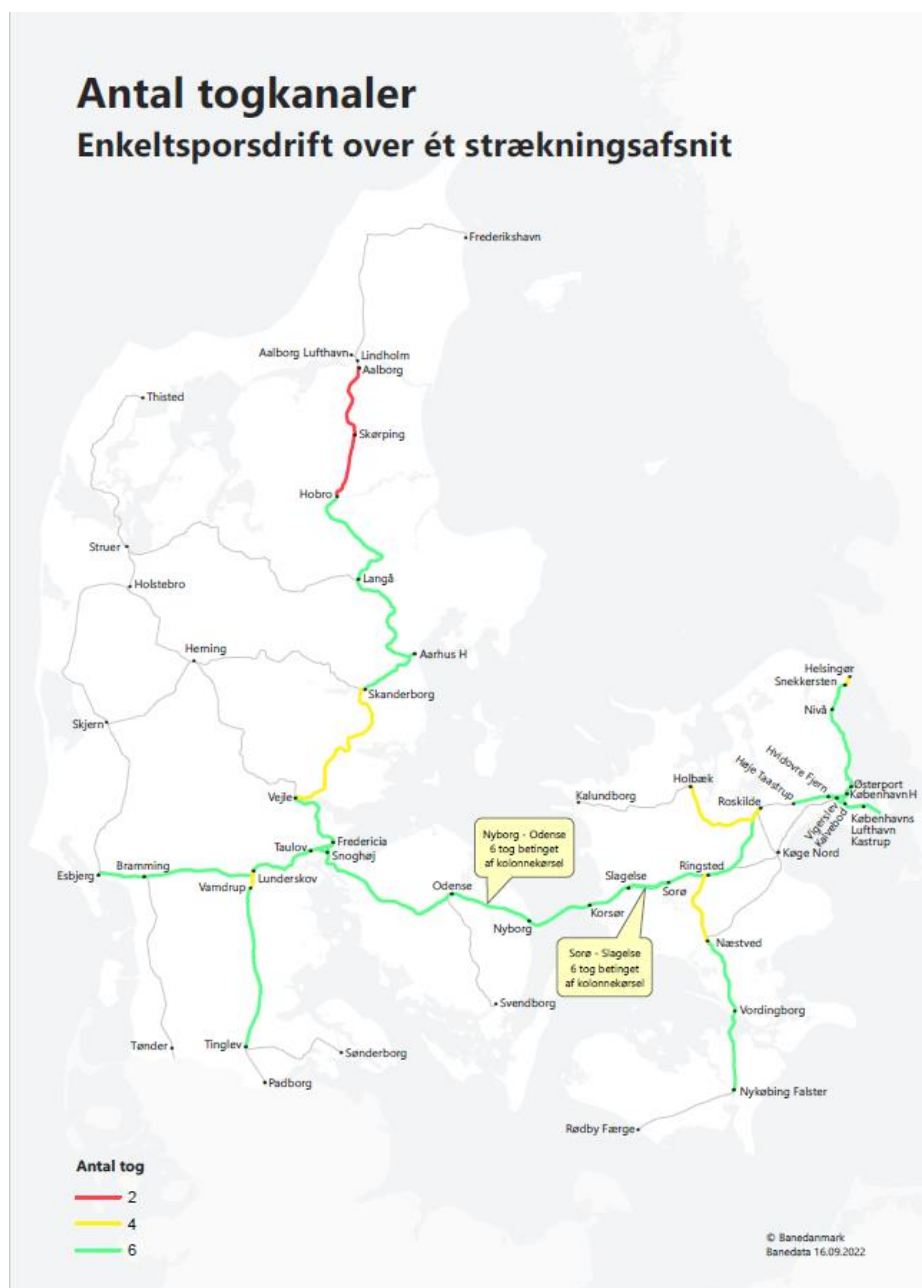
Illustration 2.1: Expected capacity during single track closures.
